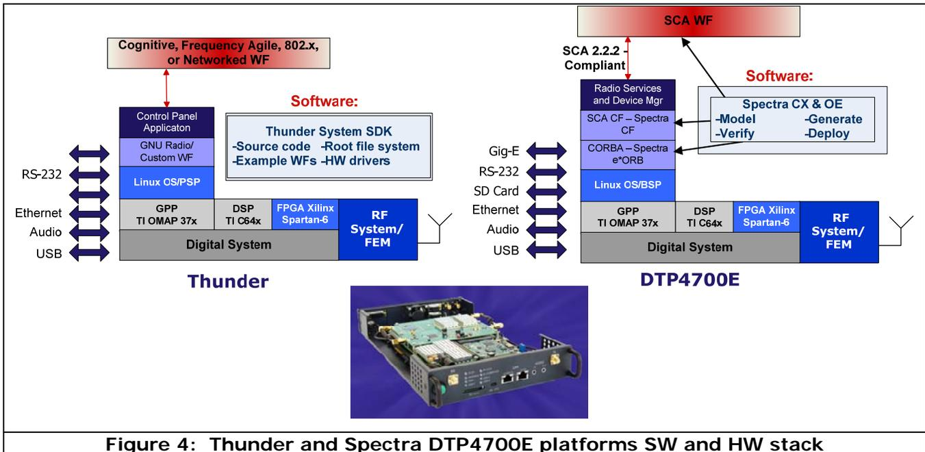
Figure 4: Thunder and Spectra DTP4700E platforms SW and HW stack
