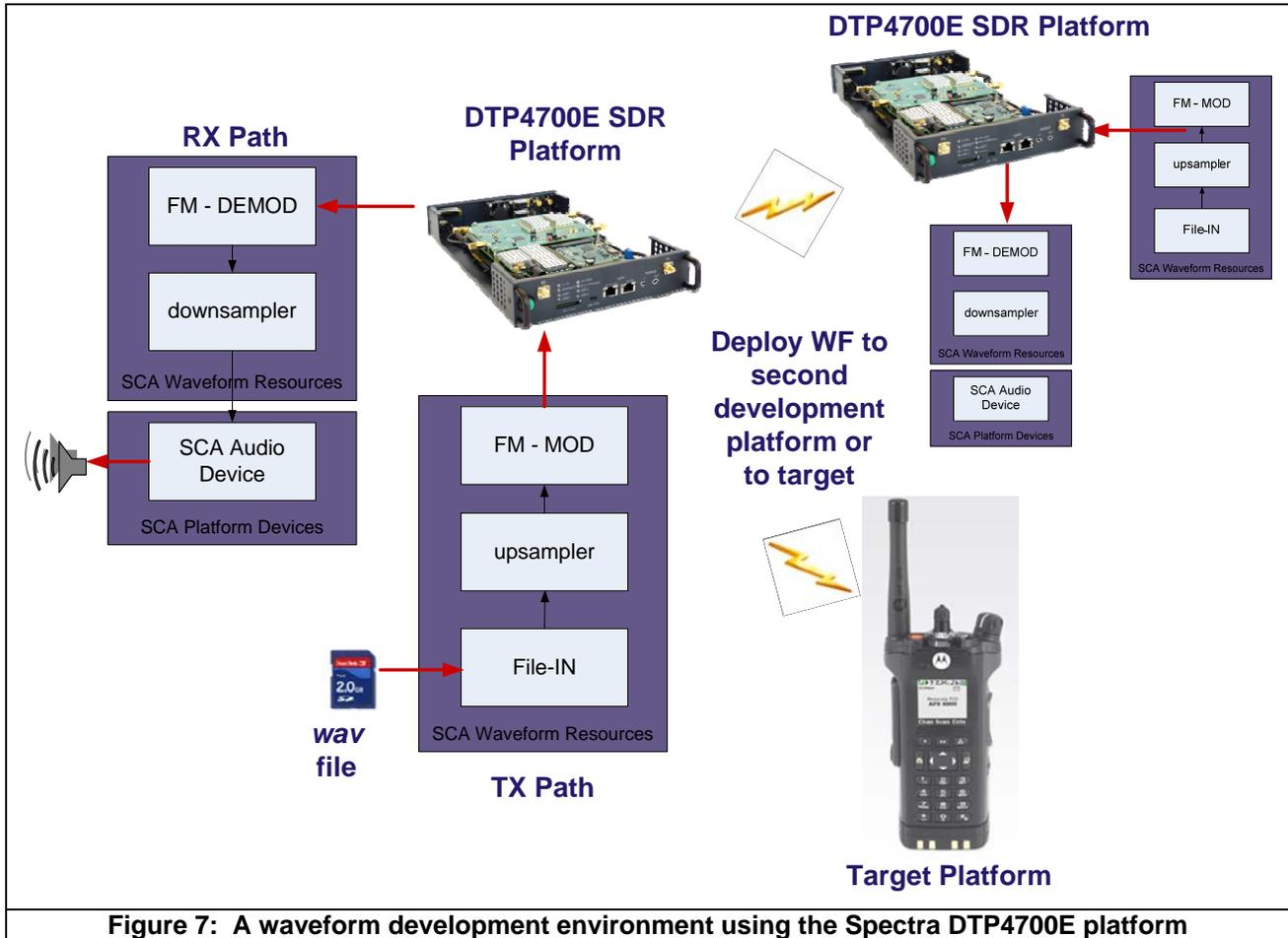
Figure 7: A waveform development environment using the Spectra DTP4700E platform
