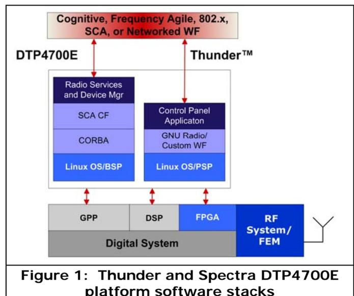
**Figure 1: Thunder and Spectra DTP4700E platform software stacks**
