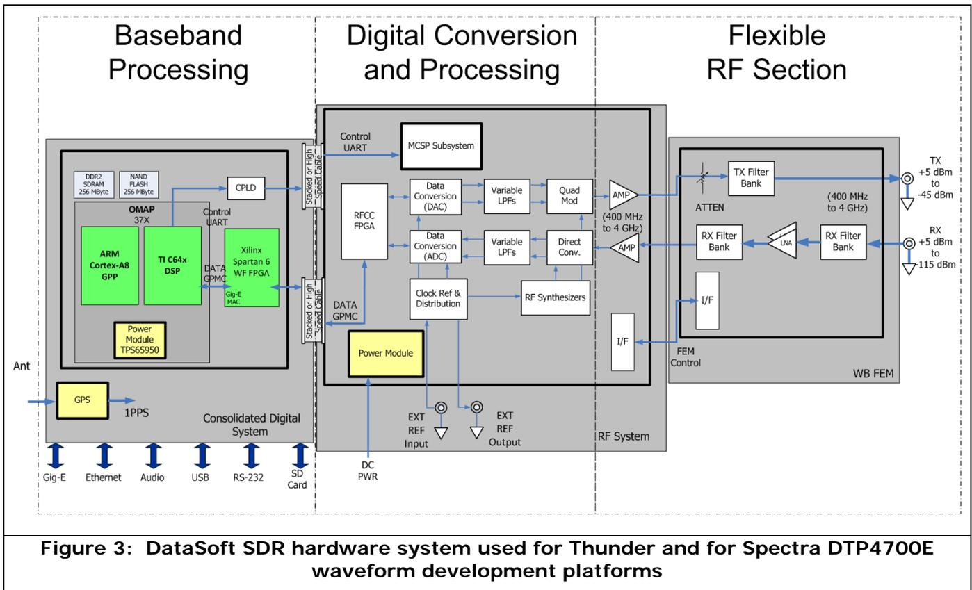
**Figure 3: DataSoft SDR hardware system used for Thunder and for Spectra DTP4700E waveform development platforms**
