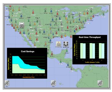
The Satellite Network Simulator Tool is used to plan satellite network expense and performance
